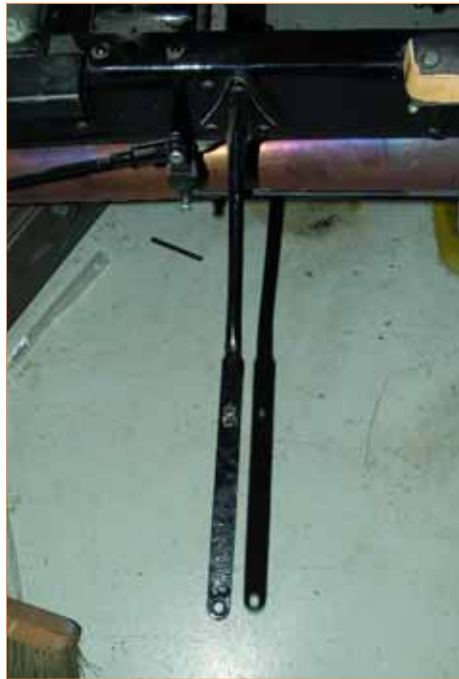
The early AR Model A Fords had many unique features that are hard to see on a completed vehicle. An example are the running board braces which are quite different than later Model A production.
